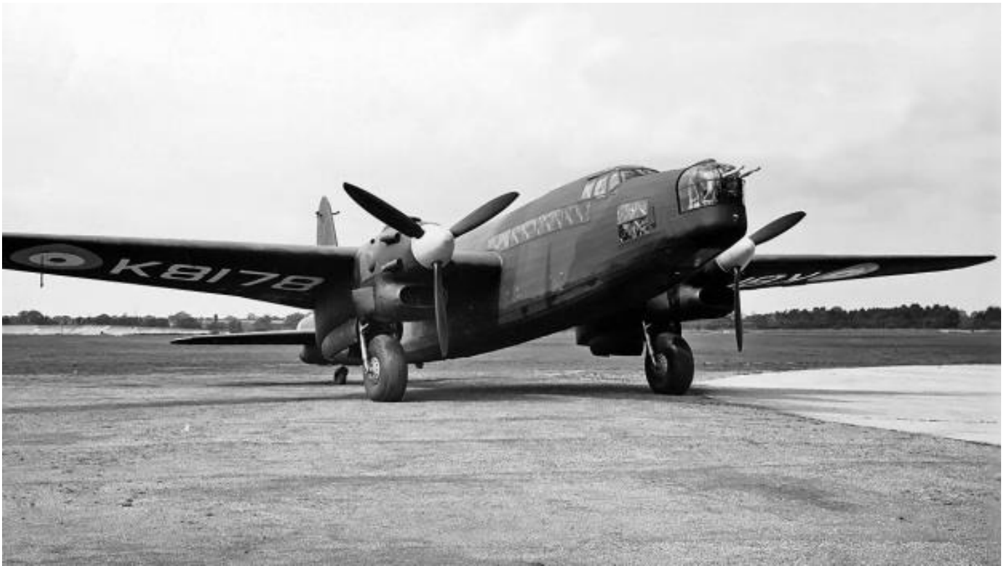
The Vickers Warwick prototype (K8178) was the only example of the type fitted with Vulture engines.
