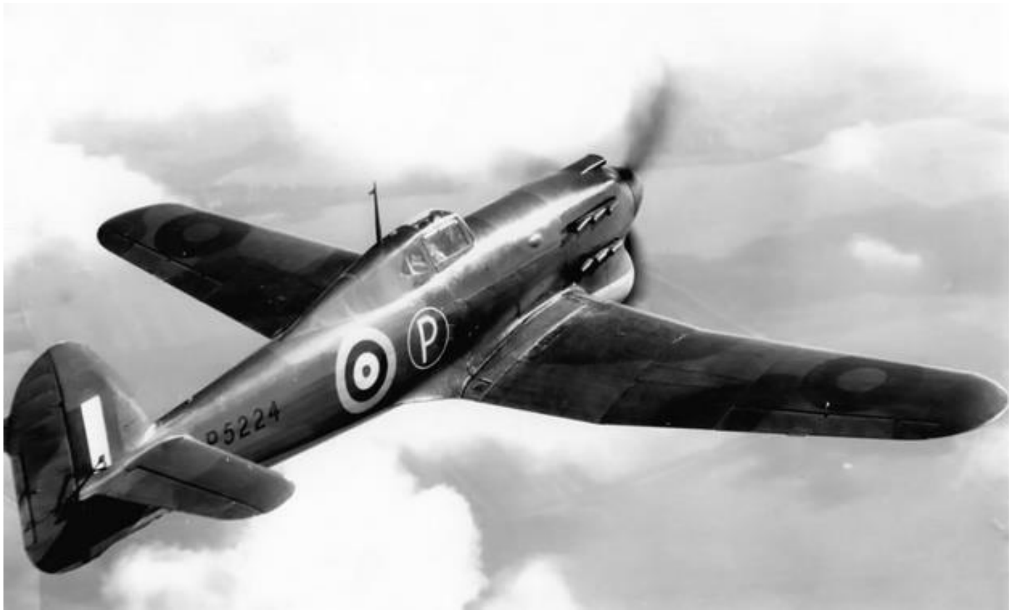
The second Hawker Tornado prototype (P5224) with its Vulture V engine. The Vulture was relatively well-behaved during testing of the Tornado, which was very similar to the Sabre-powered Typhoon.
