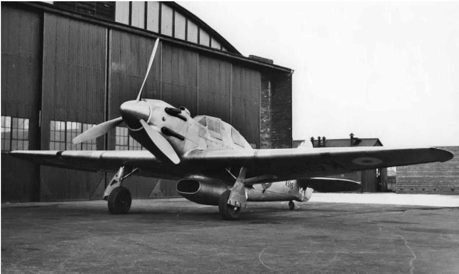
The Hawker Henley testbed (K5115) was the first aircraft to fly with a Vulture engine. The large scoop under the aircraft accommodated the coolant radiator and oil cooler.
