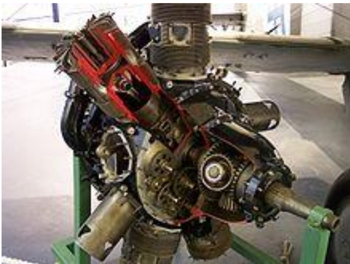
Cutaway Bristol Perseus showing sleeve valves and reduction gears
