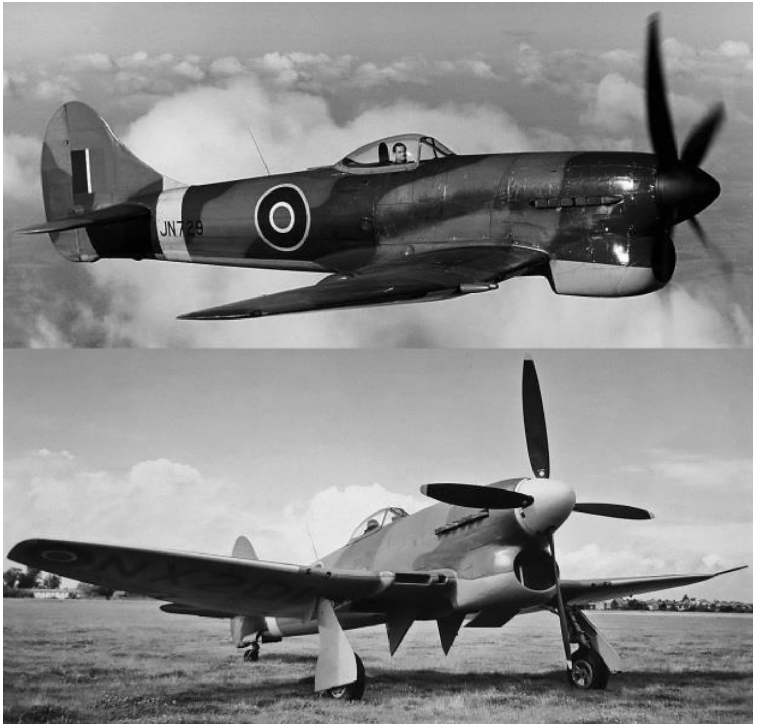
A Tempest V Series I (top) and Tempest VI (bottom). The Tempest V Series I had Hispano Mk II cannons with long barrels that protruded from the wing's leading edge. The Tempest V Series II and other Tempests had Hispano Mk V cannons with short barrels. The Sabre VA-powered Tempest VI (bottom) has an enlarged chin radiator, an oil cooler in the wing, and carburetor inlets in both wing roots.
