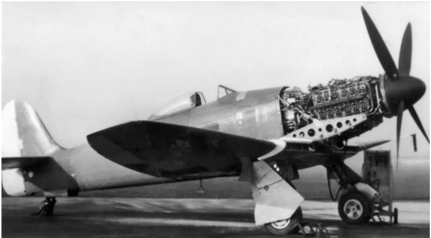
The Napier Sabre VII engine installed in the nearly-complete Hawker Fury Mk I prototype. The aircraft and engine combination created a fast and elegant fighter. Note the leading edge wing radiators. (Napier/NPHT/IMechE image)
