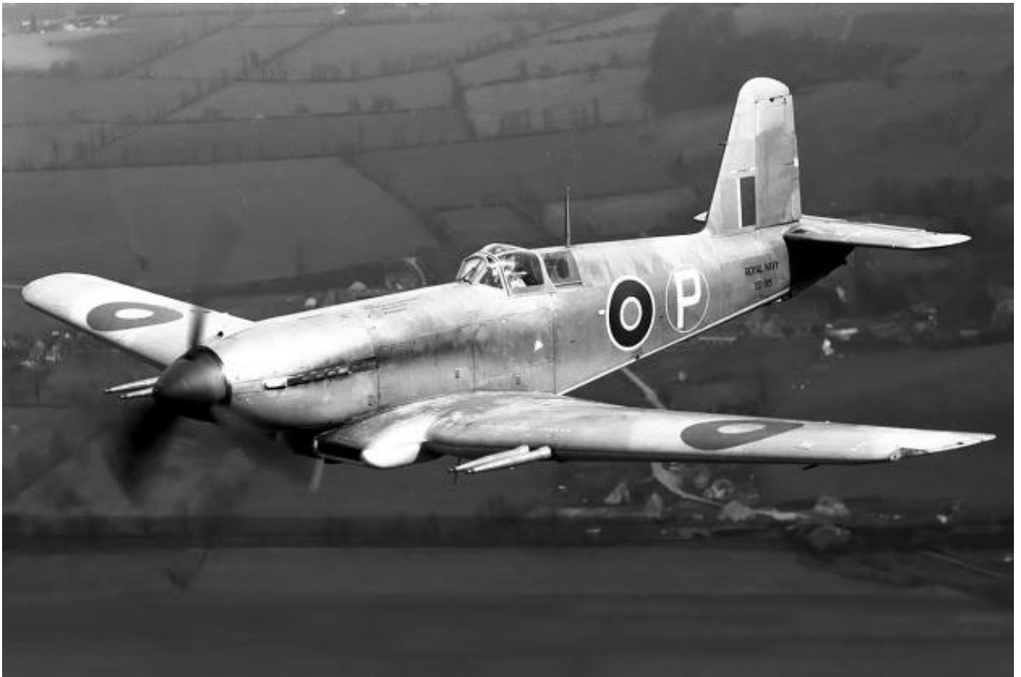
The Blackburn Firebrand, was to be powered by the Sabre III. However, Sabre engine production was allocated to the Typhoon, and the Firebrand was reengined with the Bristol Centaurus. Pictured is DD815, the third Firebrand Mk I prototype.
