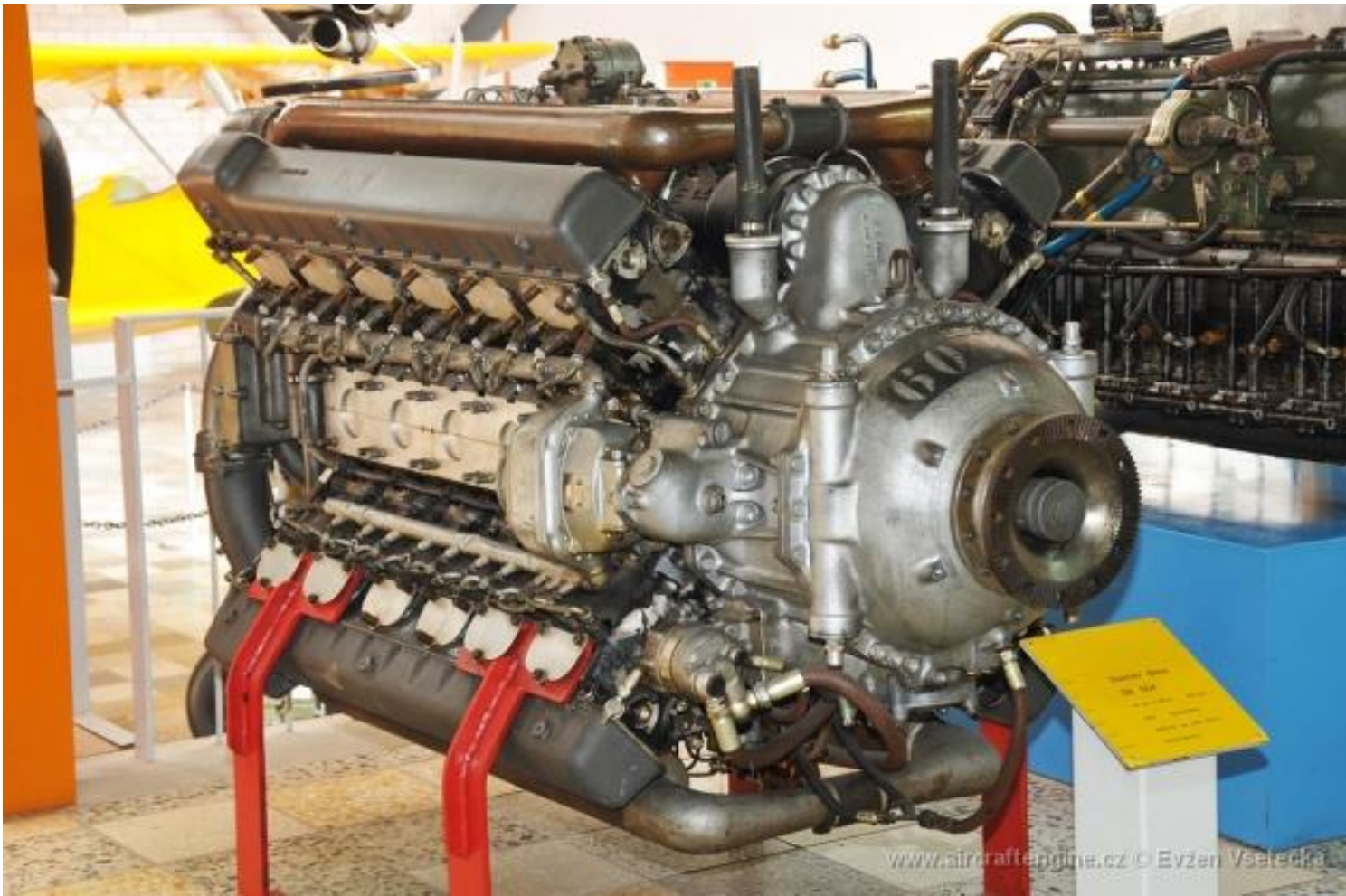
Some of the fuel injection equipment is just visible in the engine's upper Vee. The sole surviving DB 604 engine is on display at the Flugausstellung L. + P. Junior museum in Hermeskeil, Germany. (Evžen Všeček image via www.aircraftengine.cz )
