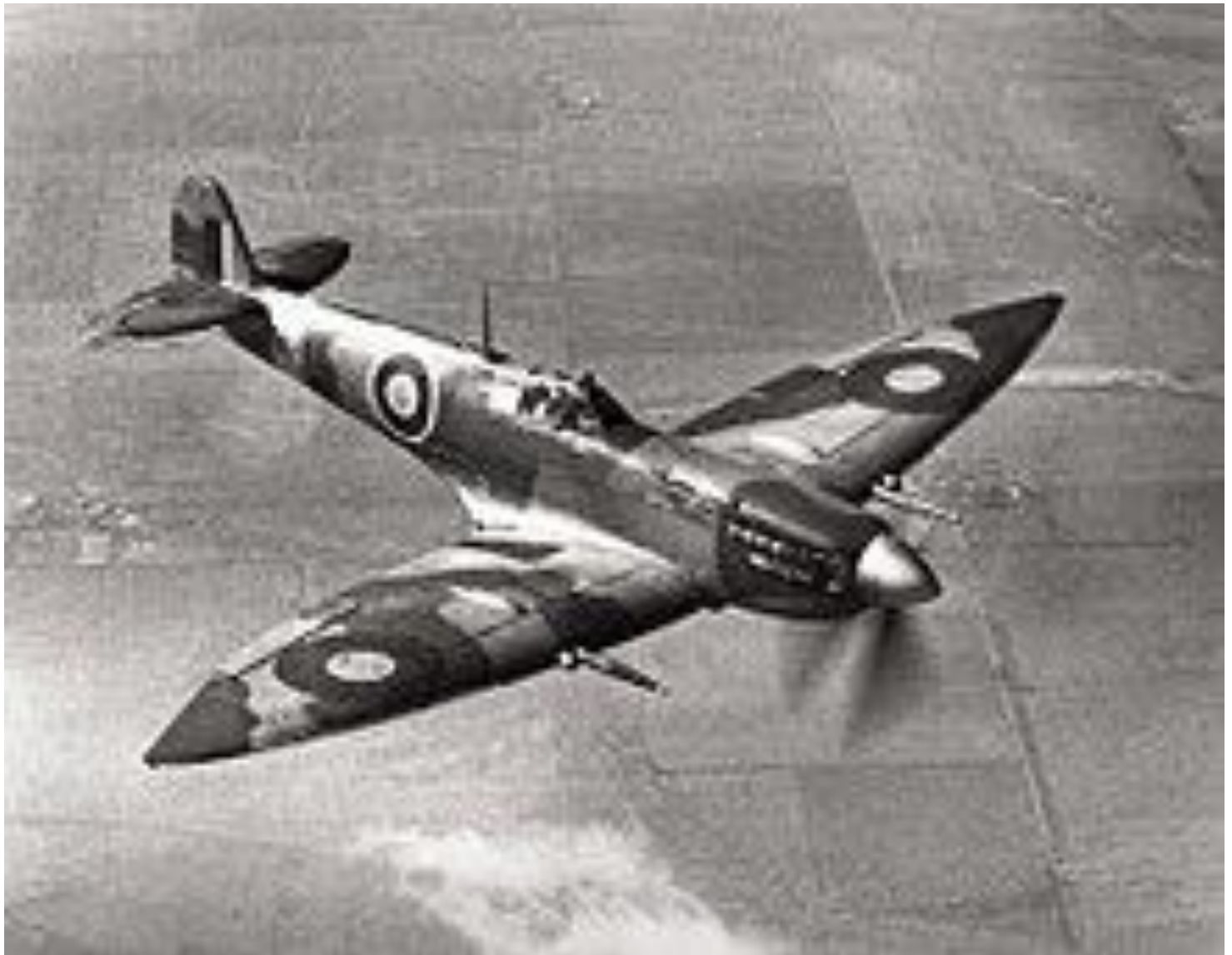
Spitfire HF Mk VII: The shape of the ellipse was altered by the extended "pointed" wing tips used by the high-altitude Mk VIs, VIIs, and early Mk VIIIs.
