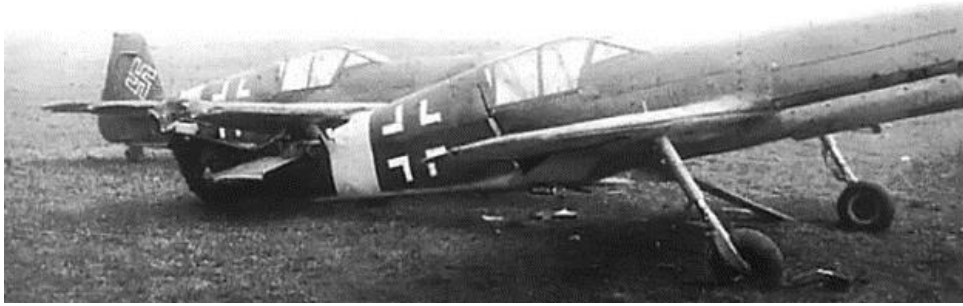
Two production Škoda-Kauba SK 257 come to grief. Note the different tail and canopy when compared to the prototype and the absence of gear doors.
