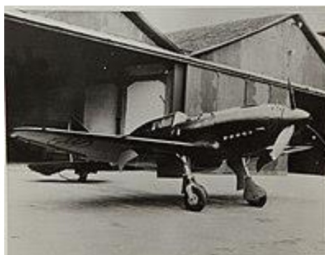
Re.2005 prototype photographed at the factory, spring 1942; note the lack of a radio mast behind the cockpit
