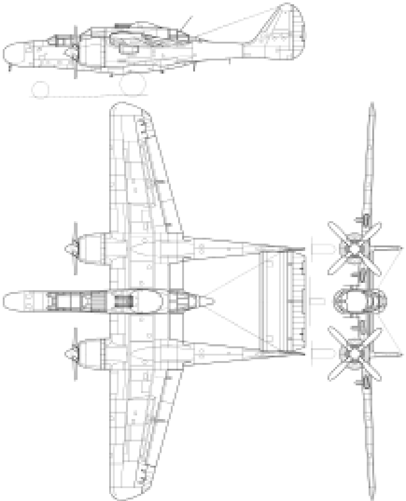
Northrop P-61B Black Widow 3-view drawing
