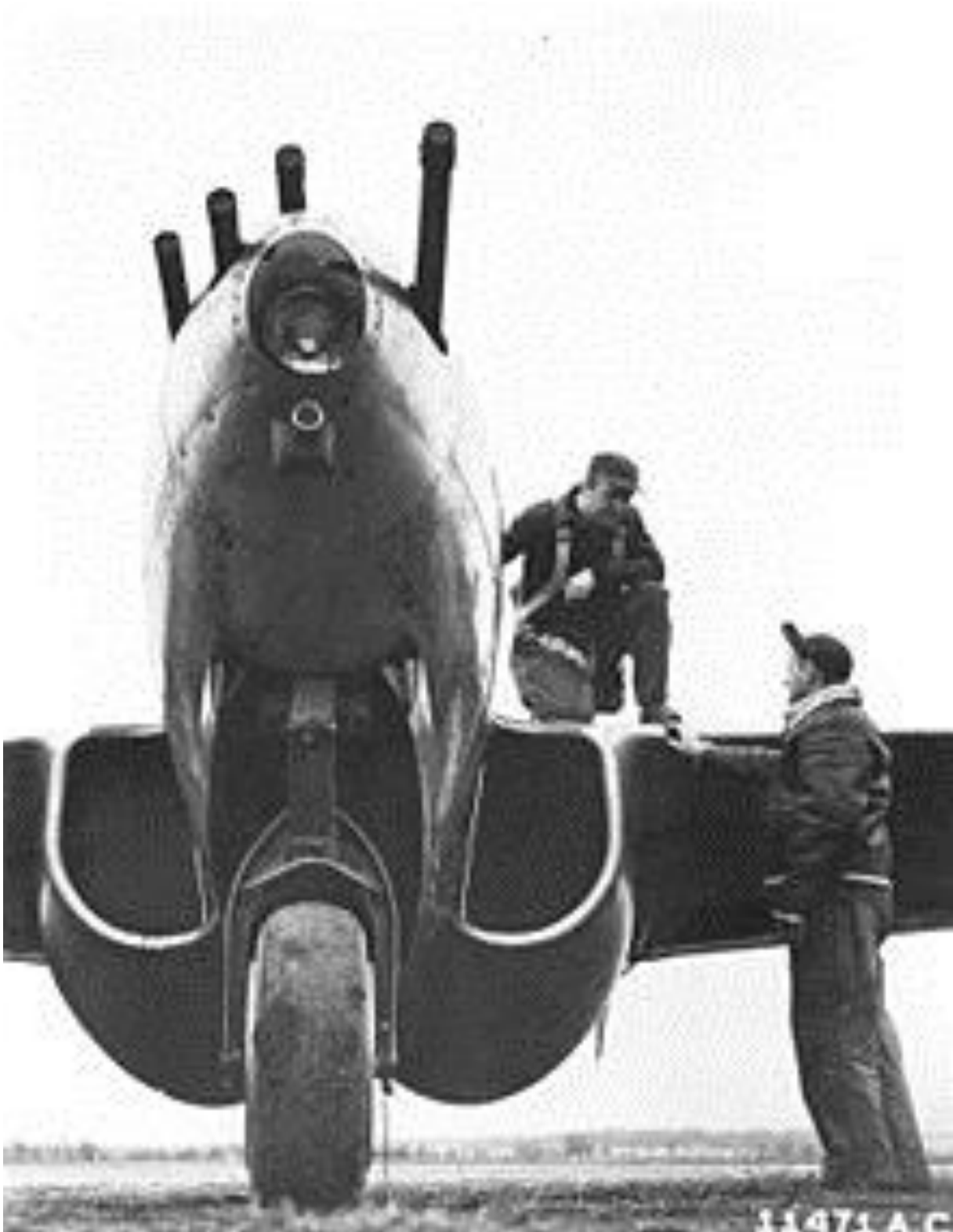
Details of fuselage and undercarriage of a P-59B, showing the nose armament
