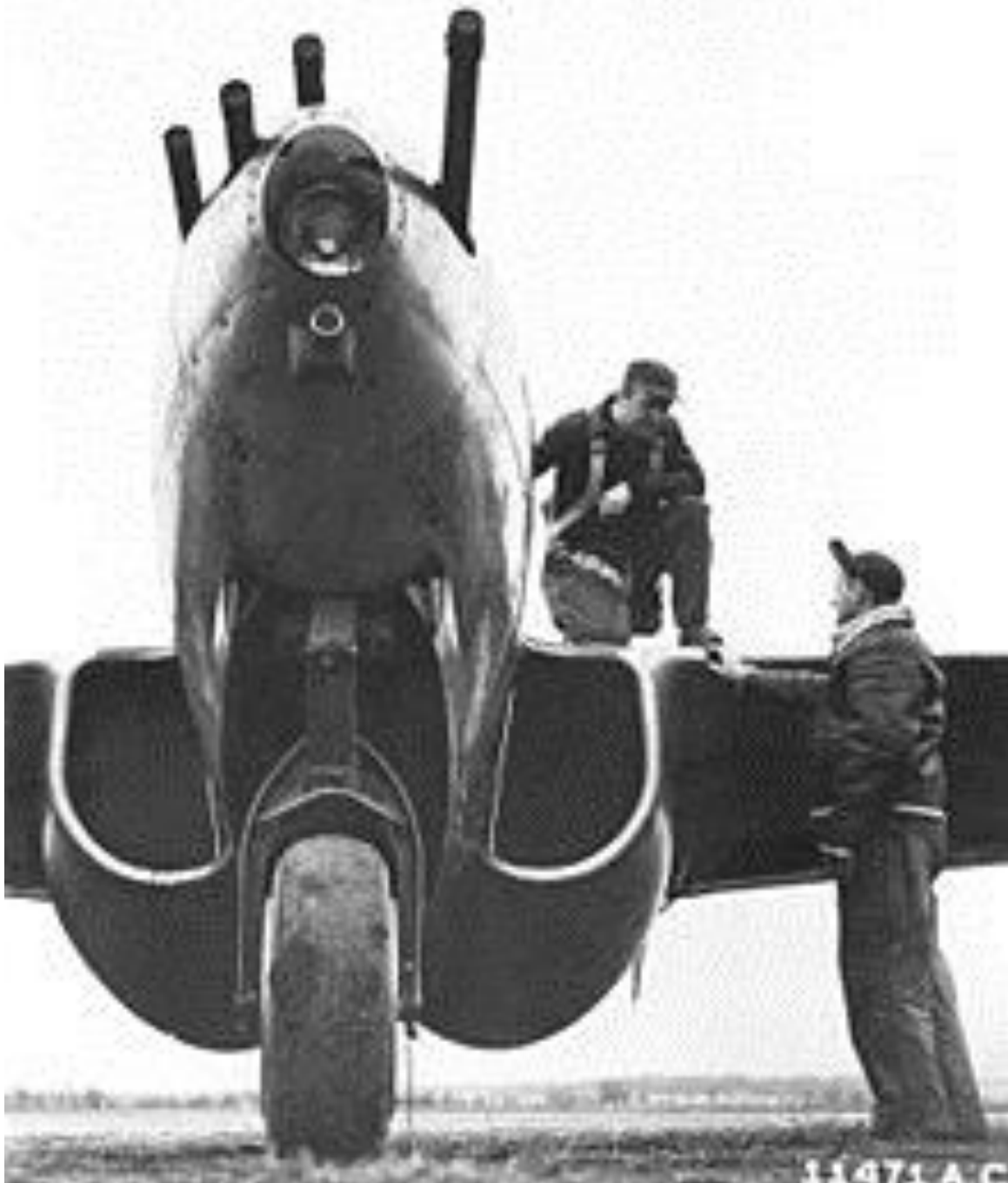
Details of fuselage and undercarriage of a P-59B, showing the nose armament
