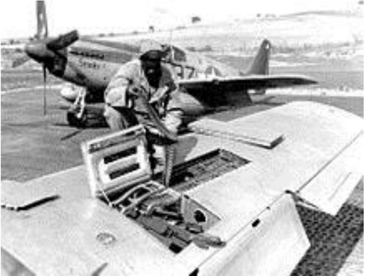
A USAAF armorer of the 100th Fighter Squadron , 332nd Fighter Group , 15th U.S. Air Force checks ammunition belts of the .50 caliber (12.7 mm) Browning machine guns in the wings of a North American P-51B Mustang in Italy, circa September 1944
