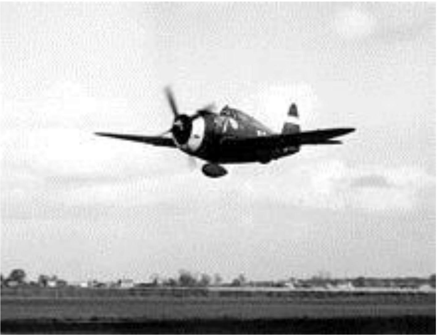
P-47D "Kathie" with a 75 US gal (62 imp gal; 284 L) drop tank buzzed the airfield at Bodney , England.
