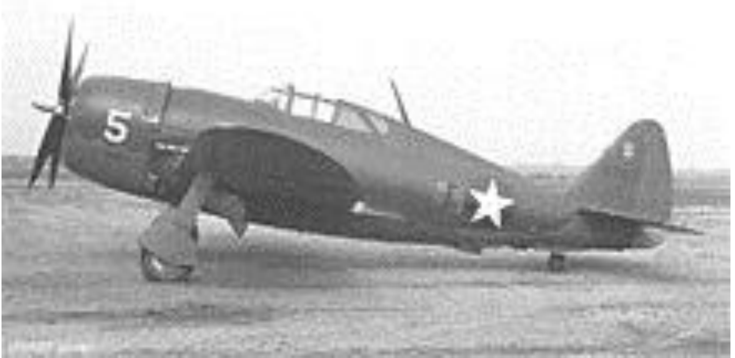
P-47B-RE 41-5905 assigned to the 56th FG at Teterboro Airport: Note the windows behind the cockpit and the sliding canopy, an indication that this was an early-production P-47B.
