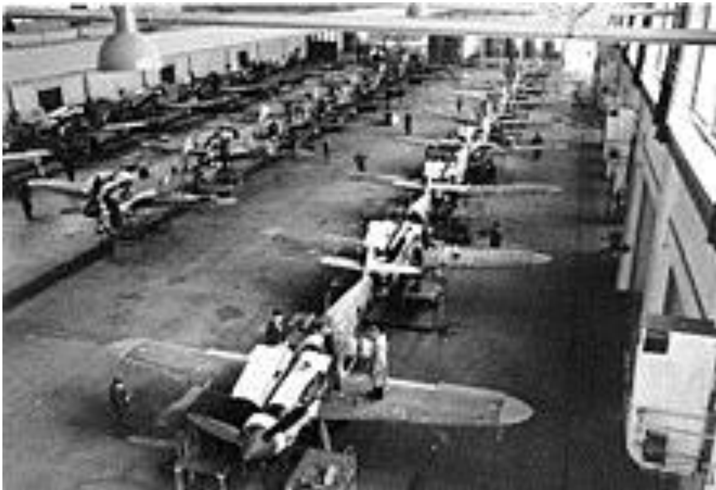
Assembly of Bf 109G-6s in a German aircraft factory.
