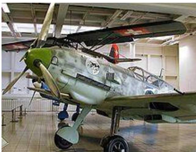
A Bf 109E-3 of JG 51 'Mölders' showing the 20 mm MG FF installations in the wing.
