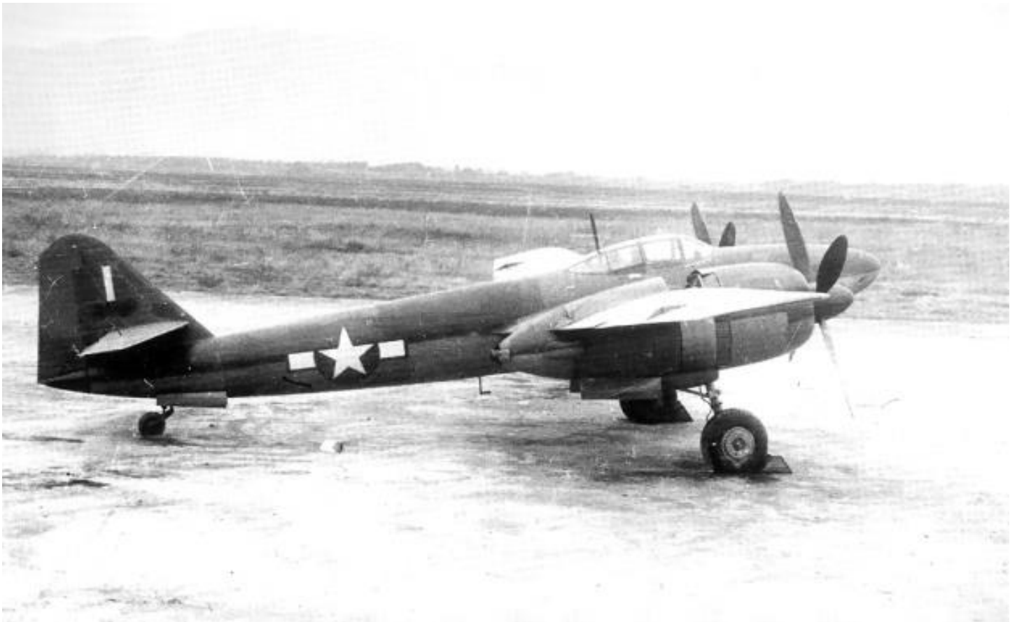
The captured Ki-83 while still in Japan. The wastegate exhaust is visible at the rear of the nacelle, and the air intake can be seen on the outboard side of the nacelle just below the trailing edge of the wing.
