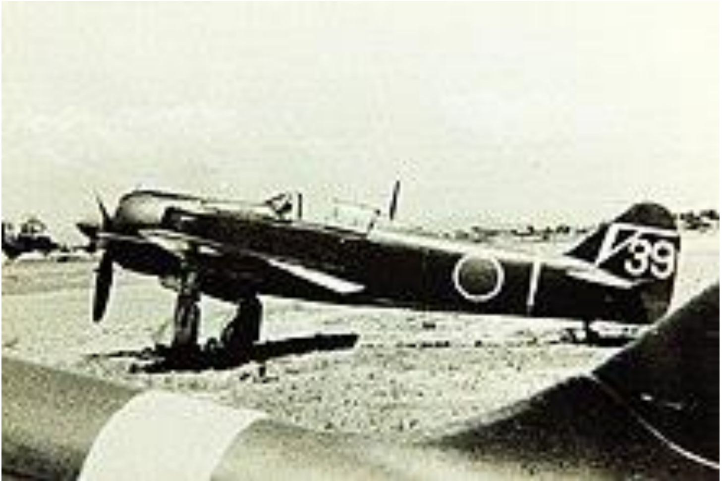
5th Sentai Ki-100-I-Otsu Army Fighter Type 5 Mark 1b, showing cut down rear fuselage
