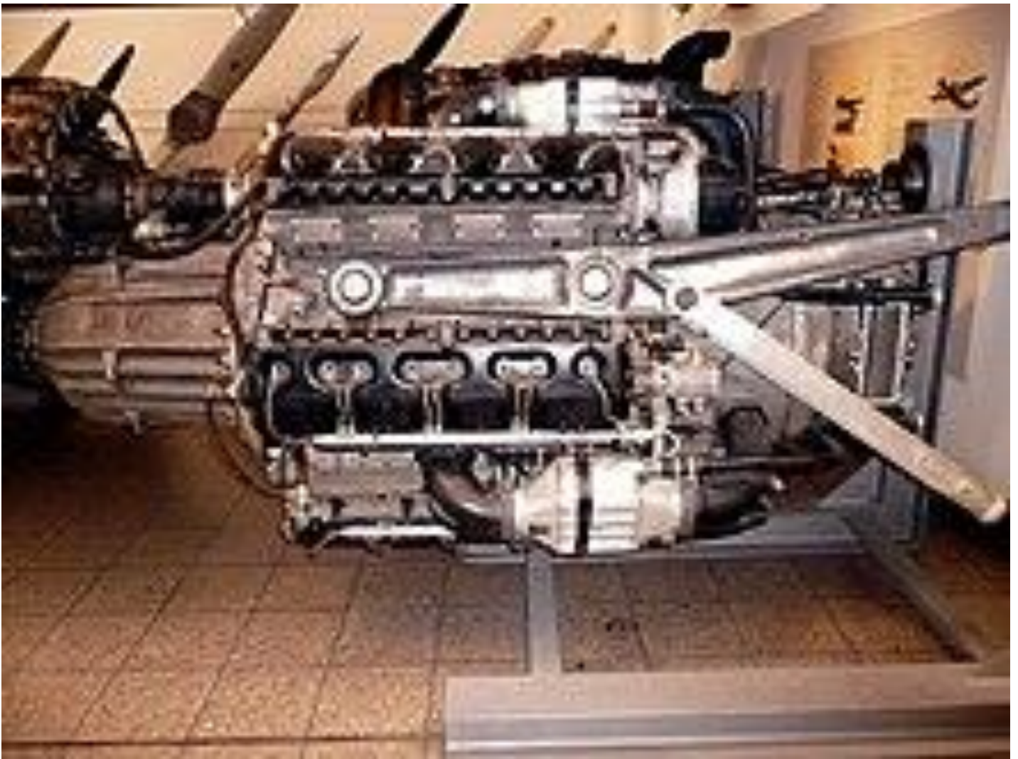
Portside view of a preserved Jumo 222E engine, intended for the Ju 388J-2 through L-2
