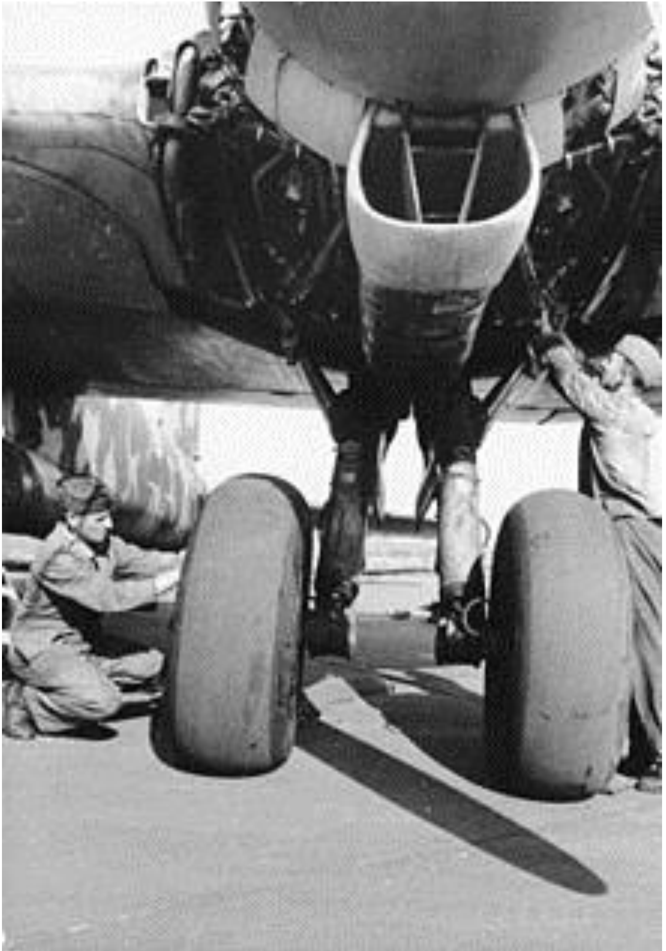
Closeup of the He 177 A's portside twin-strut main landing gear, also showing details of the "welded-together engines" tight engine installation from the ventral side of the cowling.
