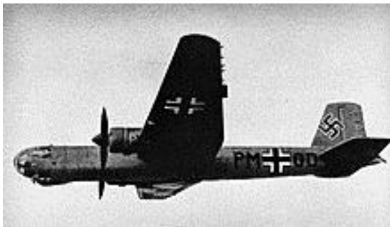
The fifth prototype He 177, the V5, with Stammkennzeichen code "PM+OD" and early cockpit design used on the first eight prototypes.
