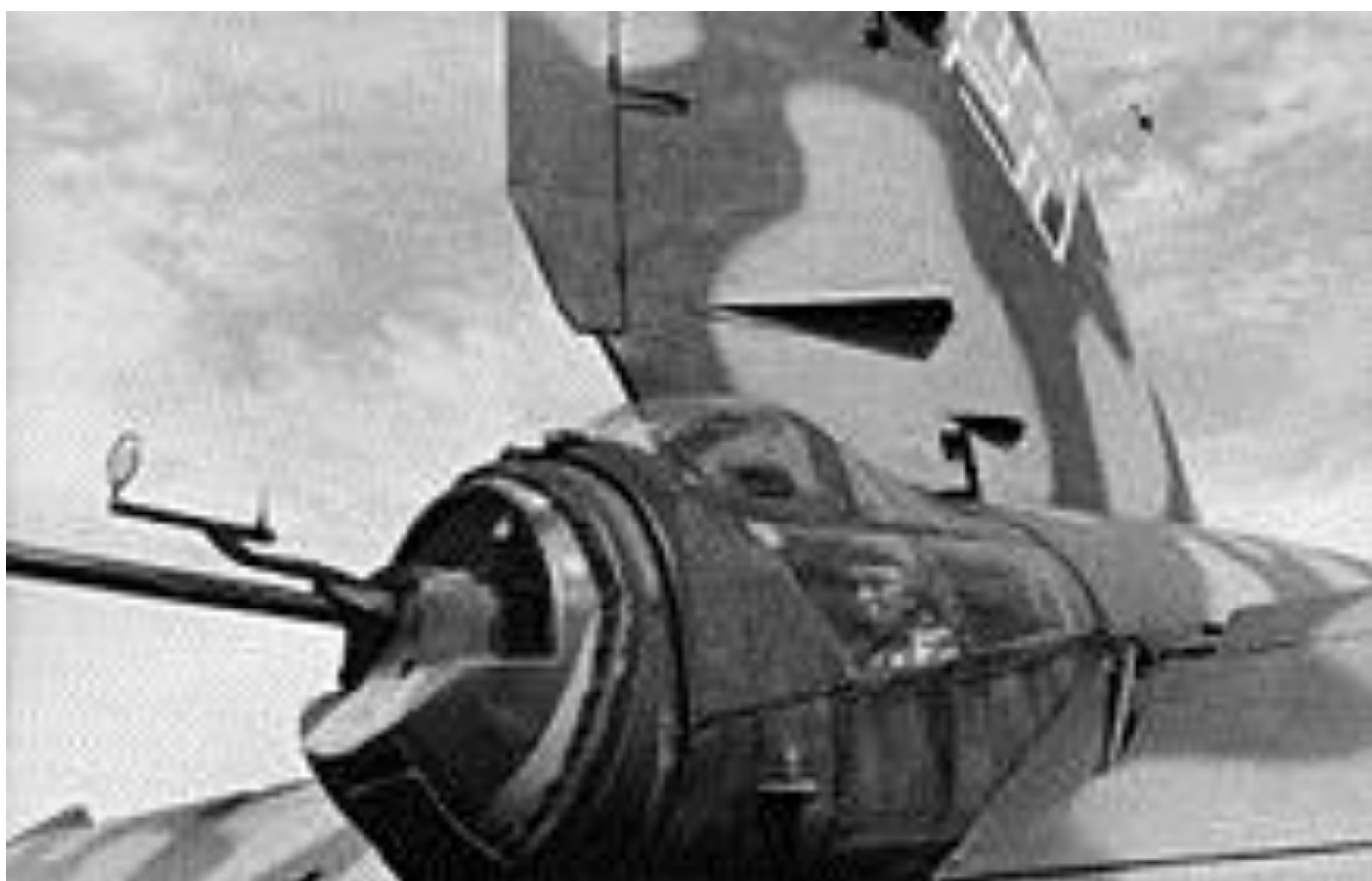
He 177 A-5 tail gun position, with MG 151 cannon and bulged upper glazing for upright gunner's seating.
