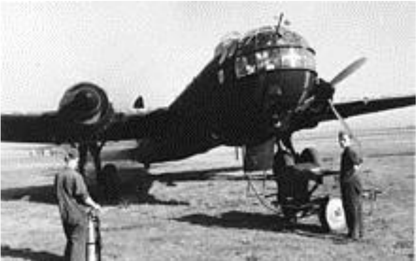
An He 177 during refueling and engine-run up 1943. Note the four-bladed propeller. The aircraft is painted in a night camouflage scheme.
