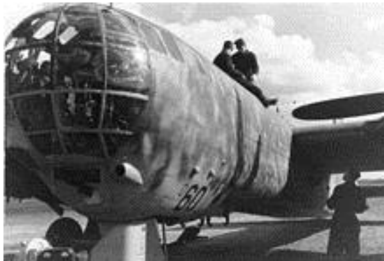
Closeup of the "fishbowl" nose glazing and Bola undernose gondola of an A-series Greif - the B-series prototypes (V101-V104) used them as well.
