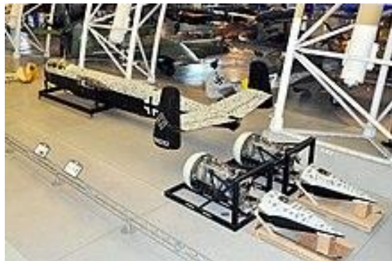
The NASM's partly restored He 219 A-2 with its unitized DB 603 engines and fuselage.
