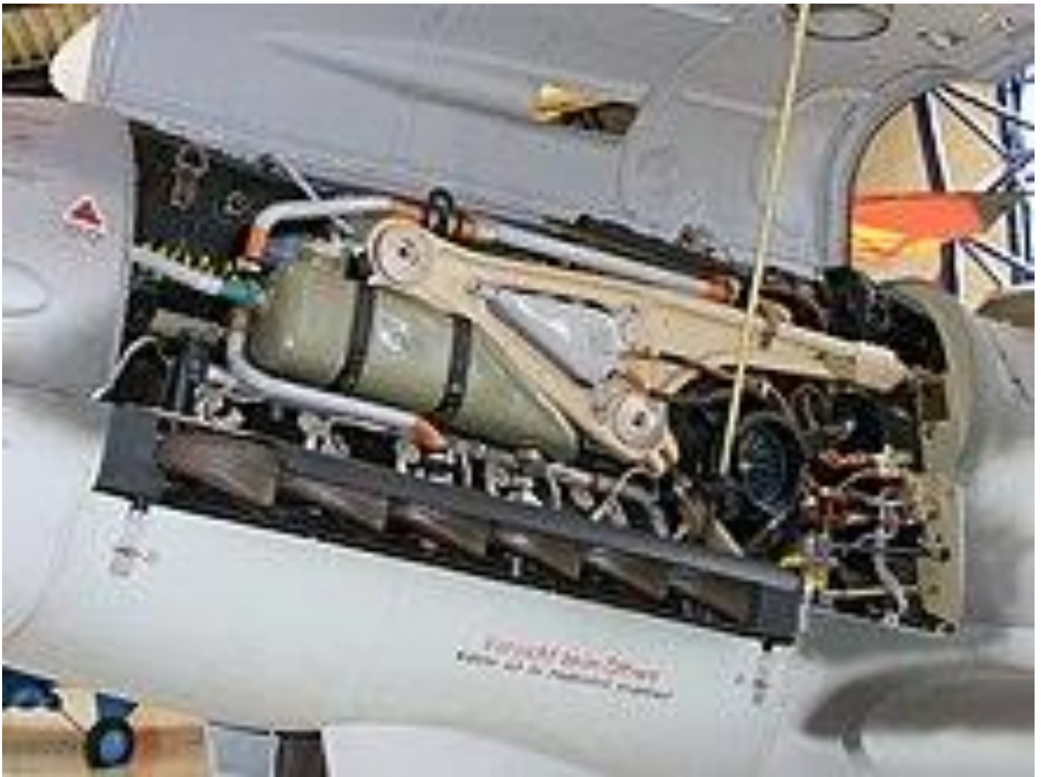
Portside view of a DB 605 engine in a Bf 109 G's nose - the visible engine mount forging was similar to what each side of the DB 606/610 used, along with the "power system's" special centreline mounting unit.
