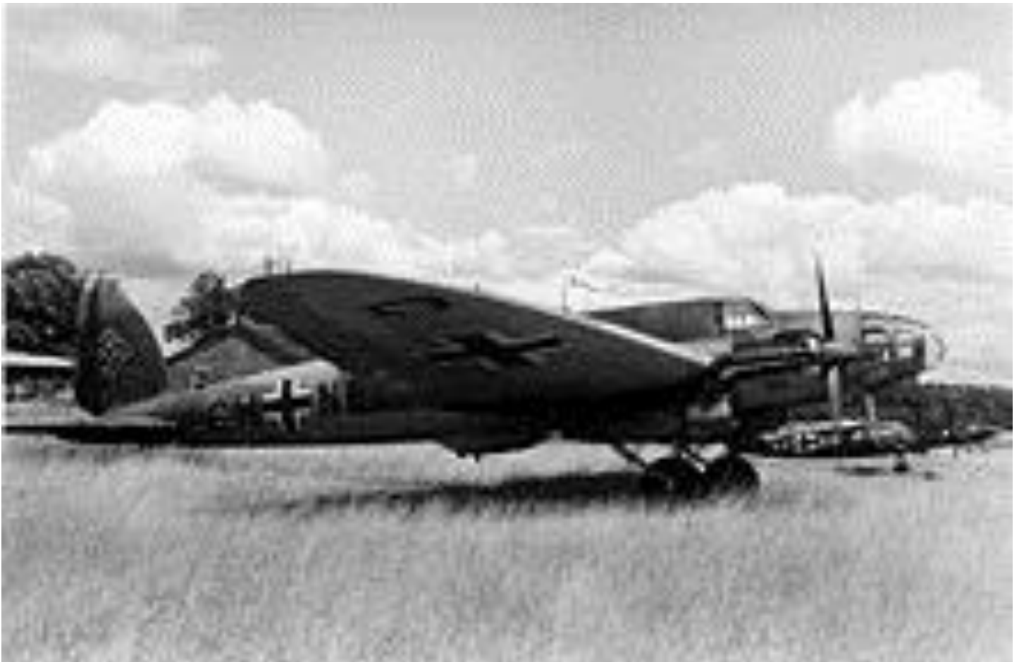
An He 111E in Luftwaffe service, 1940. The early variants had a conventional, stepped cockpit.
