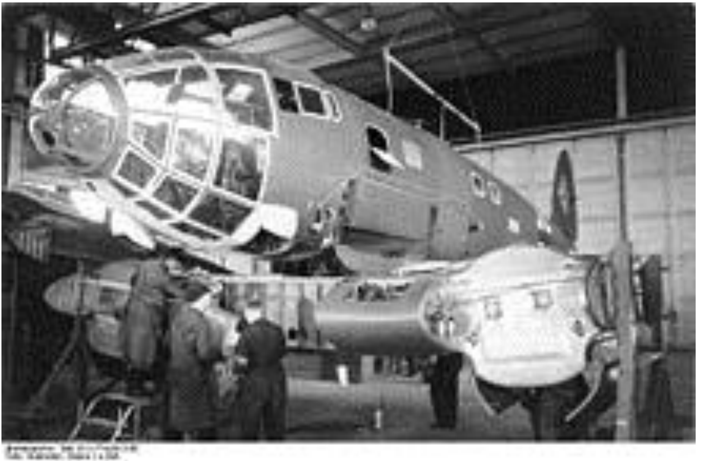
An He 111 in the preliminary stage of wing installation
