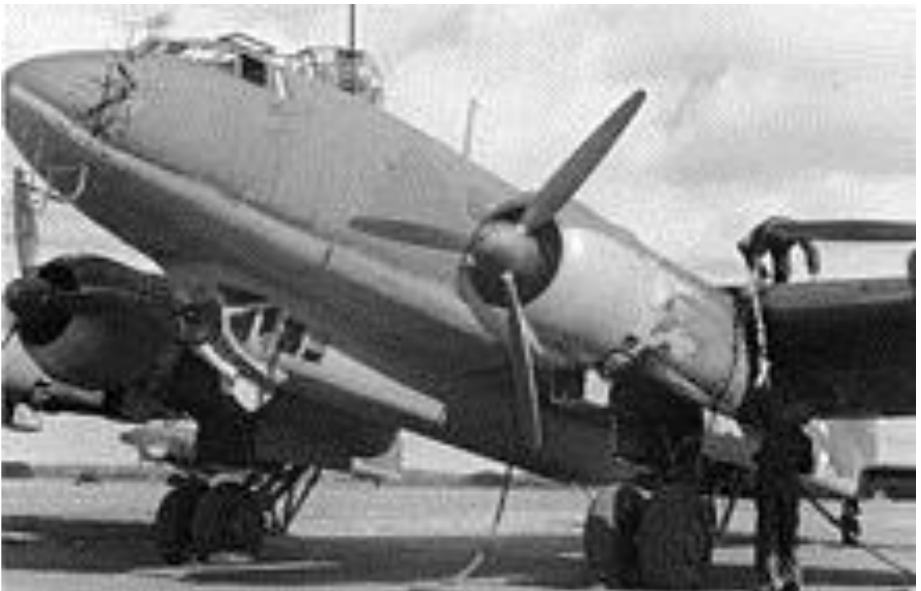
The ASV radar-equipped Fw 200 C-4, showing the twin-wheel main gear used for all production Fw 200Cs and enlarged dorsal turret of the C-3/U1
