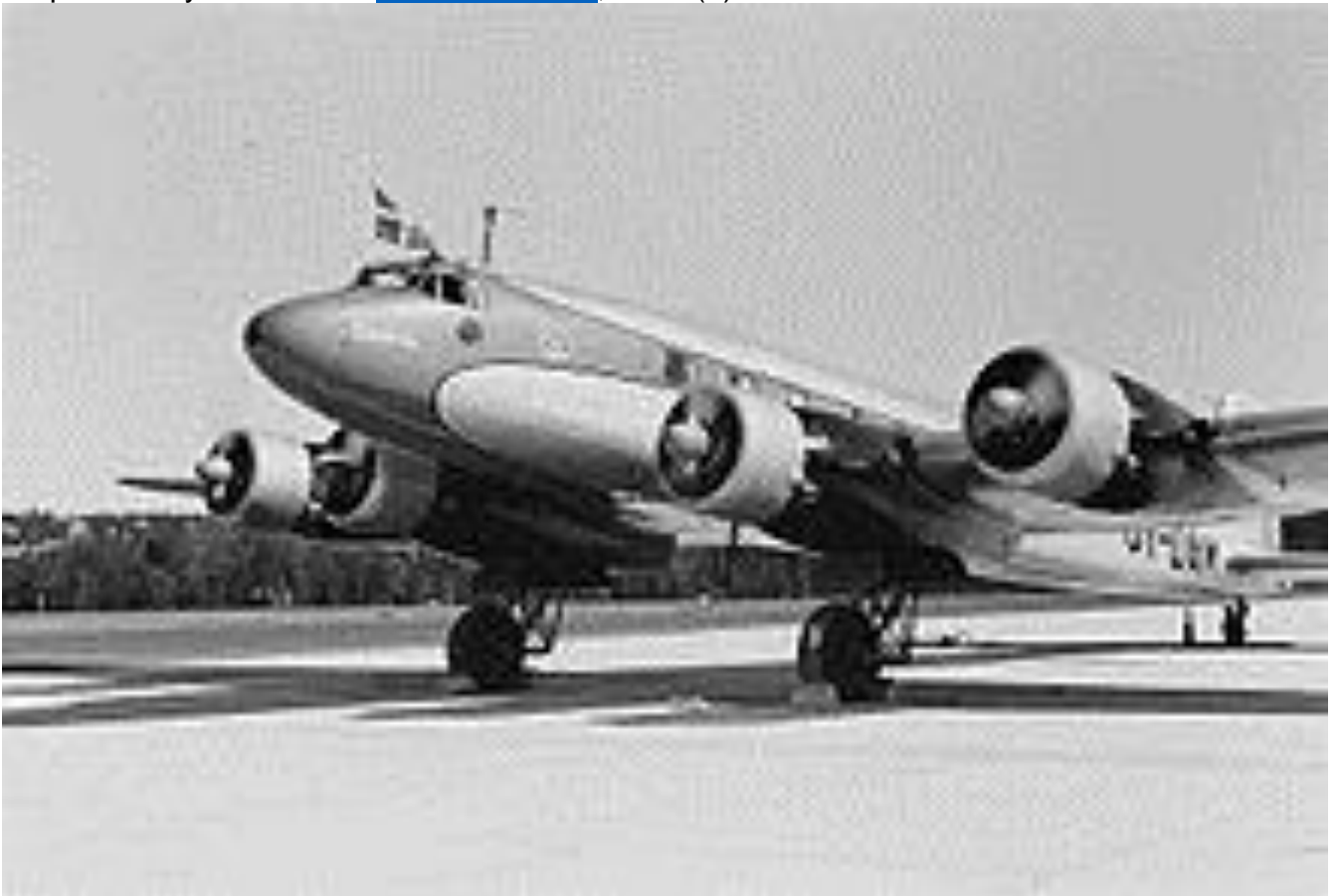
Danish Fw 200 airliner Dania at Fornebu Airport in Norway in 1939, with early single-wheel main gear.
