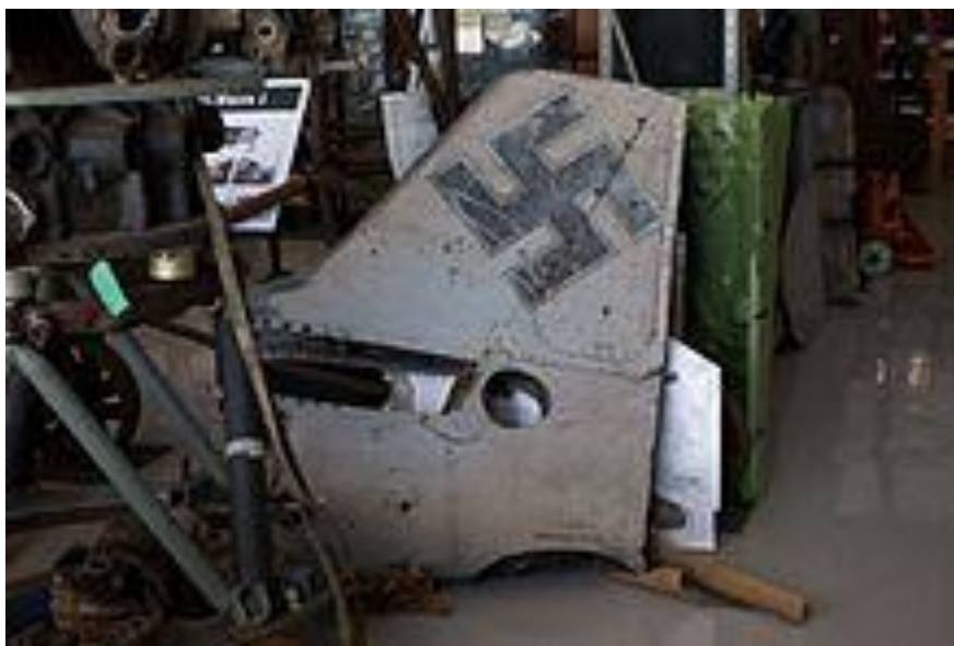
An Fw 190F's tailfin, showing the triangular hinged panel for access to the tailwheel retraction mechanism inside of it
