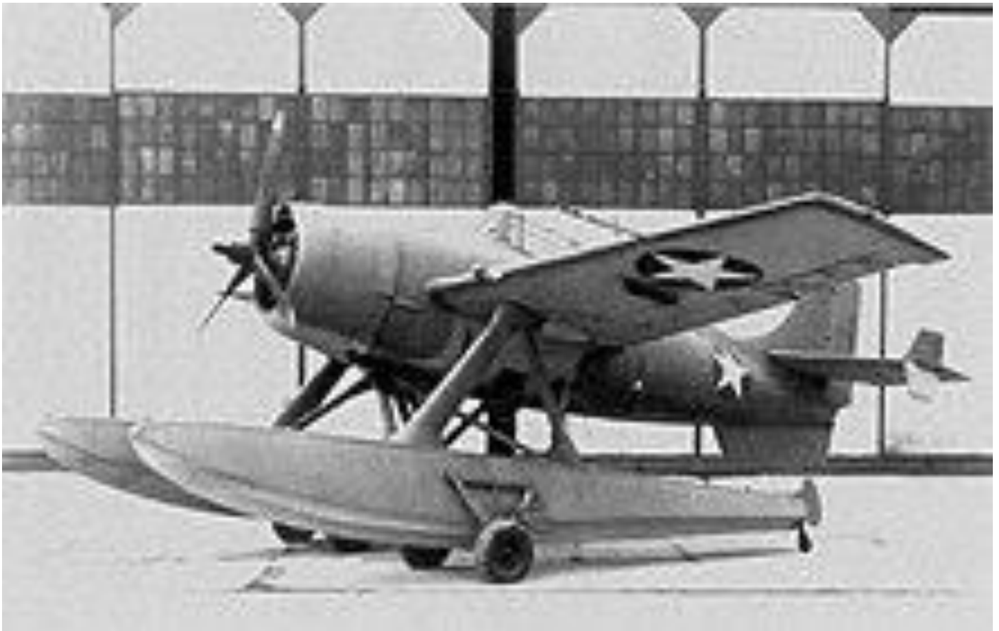
The F4F-3S "Wildcatfish", a floatplane version of the F4F-3. Edo Aircraft fitted one F4F-3 with twin floats.
