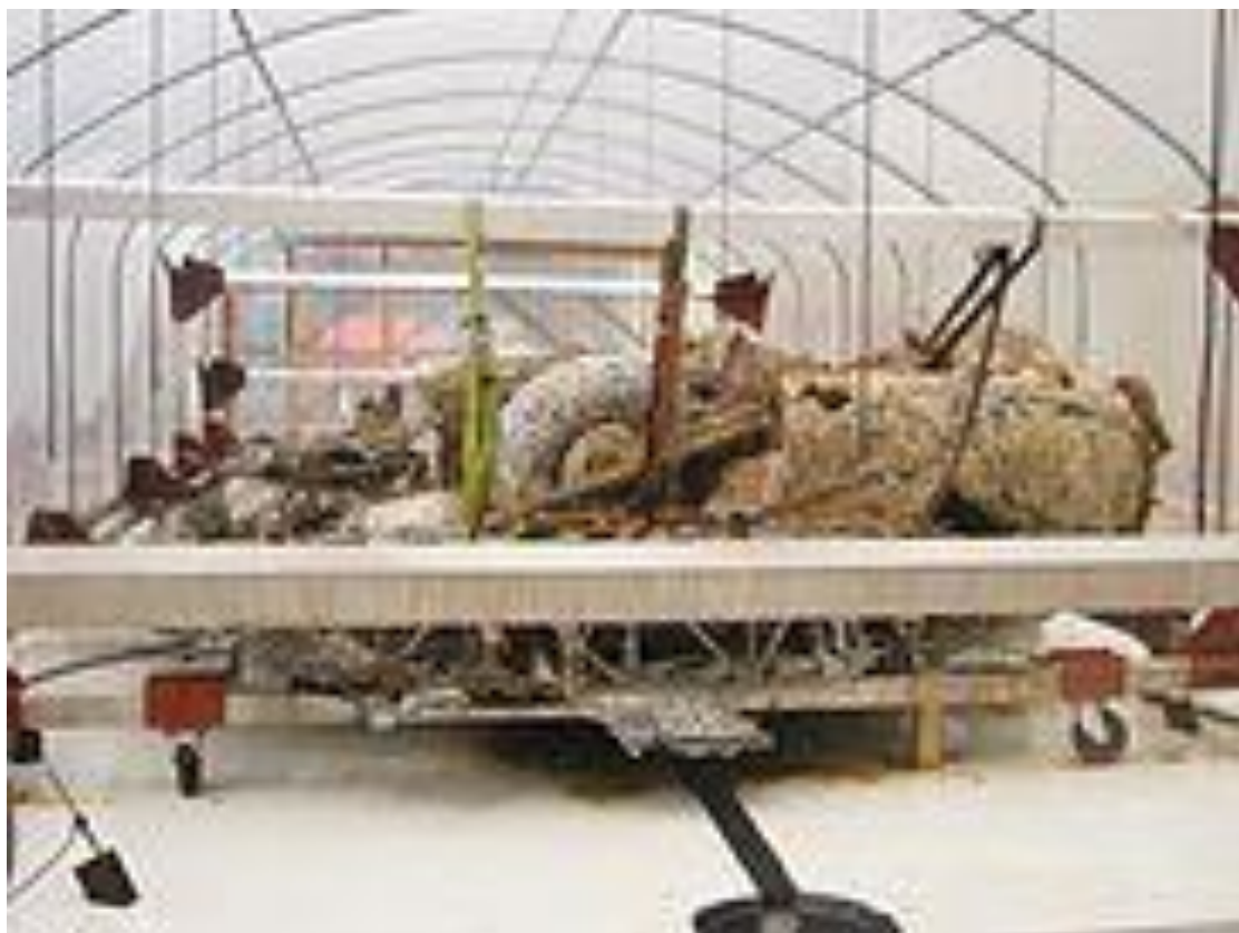
Port engine nacelle; note the tyre is still pressurized
