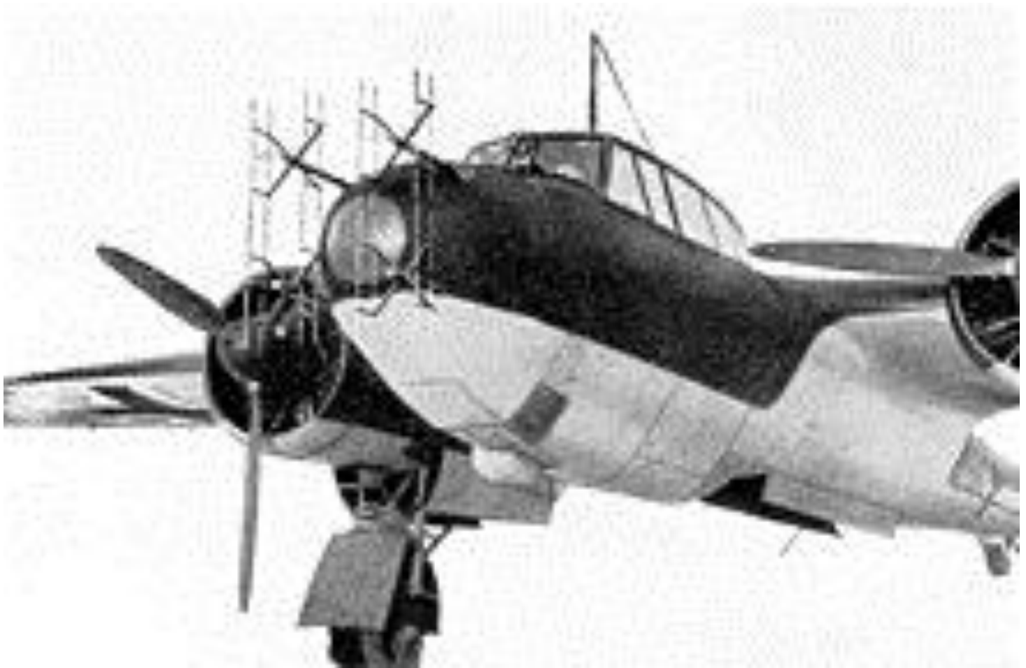
Dornier Do 17Z-10 night fighter with FuG 202 Lichtenstein B/C UHF radar
