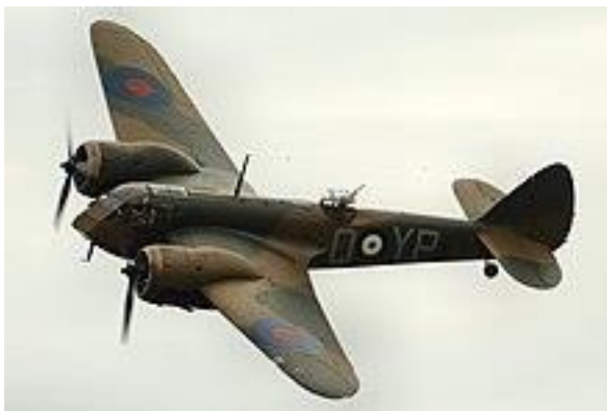
Bolingbroke IVT with an early Blenheim nose grafted on, flying at Duxford in 2015, painted as Mk.1 L6739
