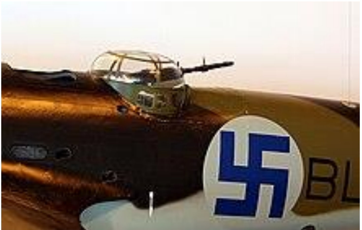
Dorsal gun turret of a Blenheim with Finnish Air Force markings
