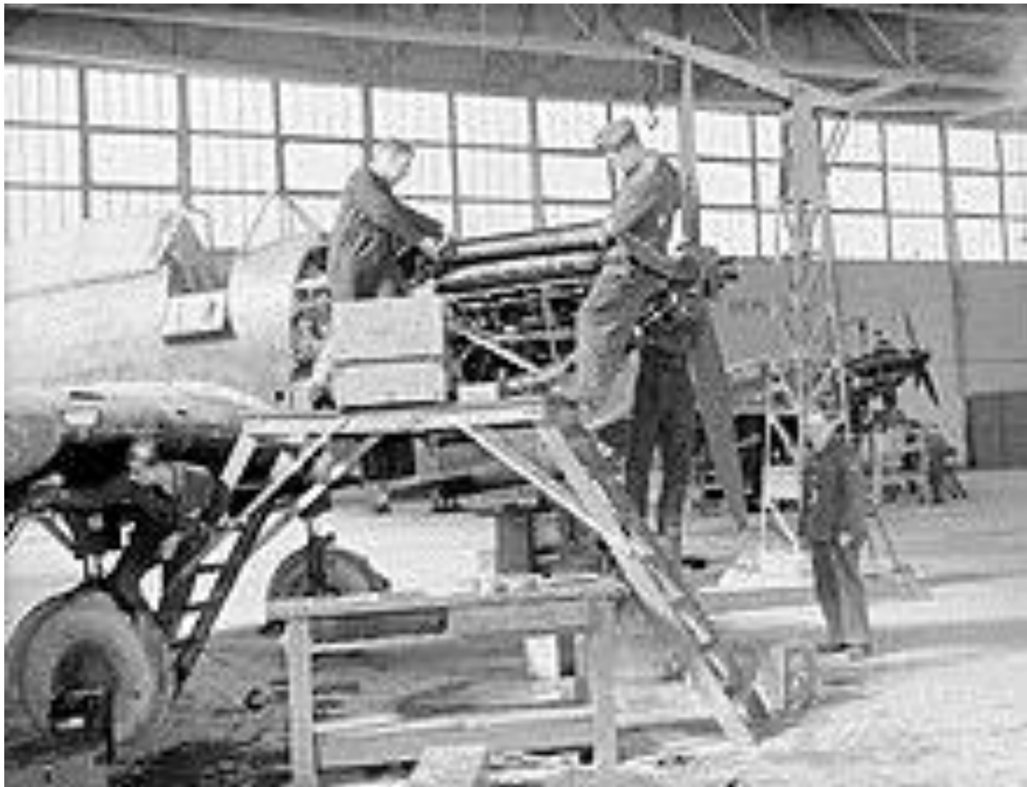
Mechanics of No. 226 Squadron RAF overhaul the engines of their Battles in a hangar at Reims , France
