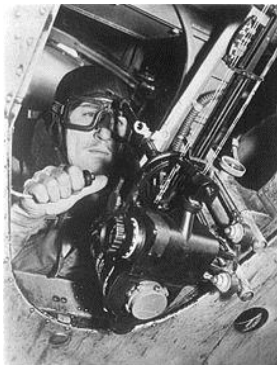
The bomb aimer position in the Battle was in the aircraft's floor. Note the CSBS Mk. VII equipment
