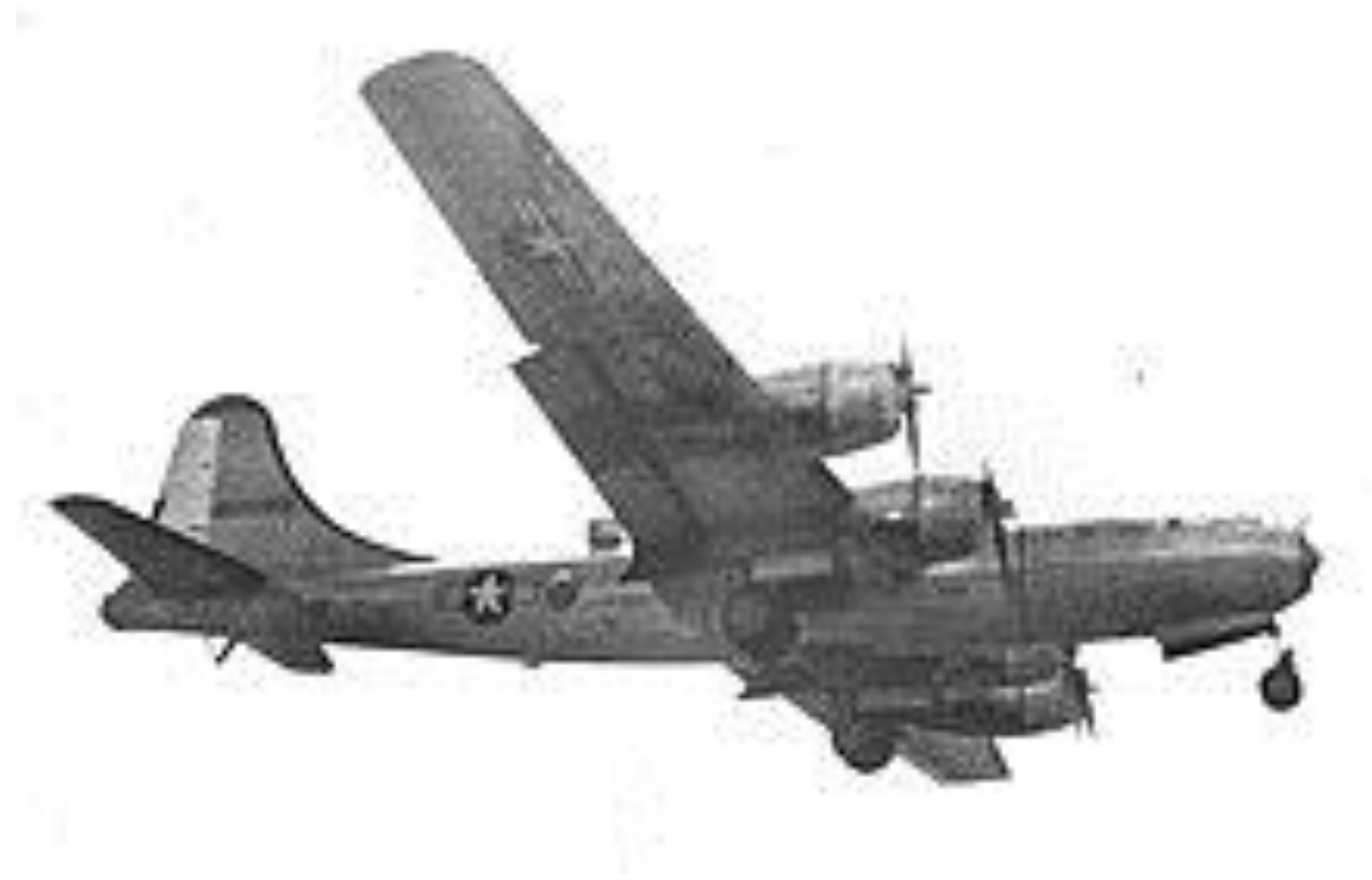
WB-29A of the 53d Weather Reconnaissance Squadron in 1954 showing the fuselage-top observation station
