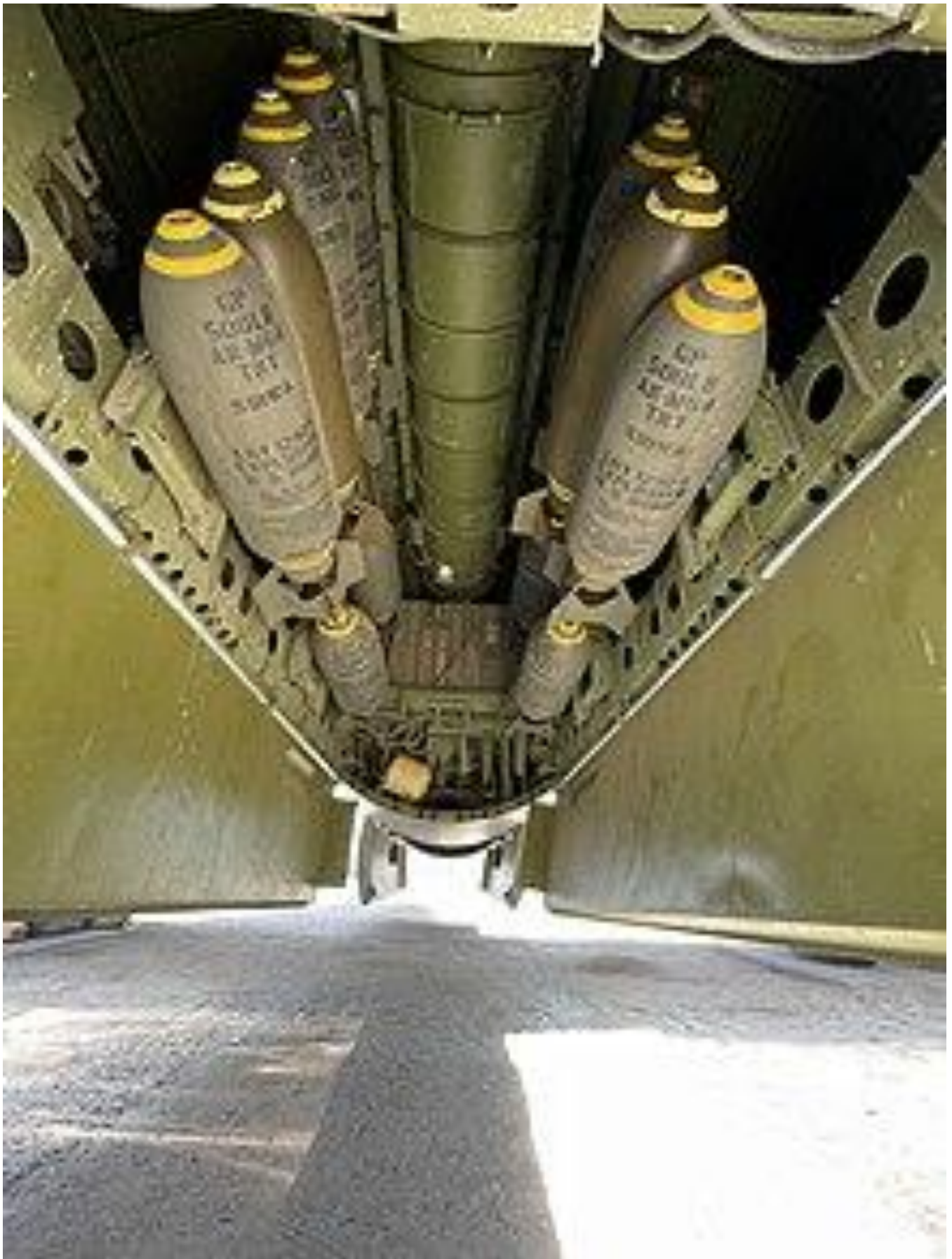
B-29 Weapons Bay with General-Purpose AN-M64 TNT 500 LB bombs
