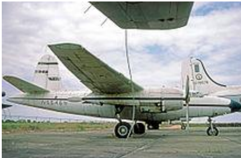
B-26C modified for corporate use in 1948 with faired nose and rear fuselage and added passenger windows
