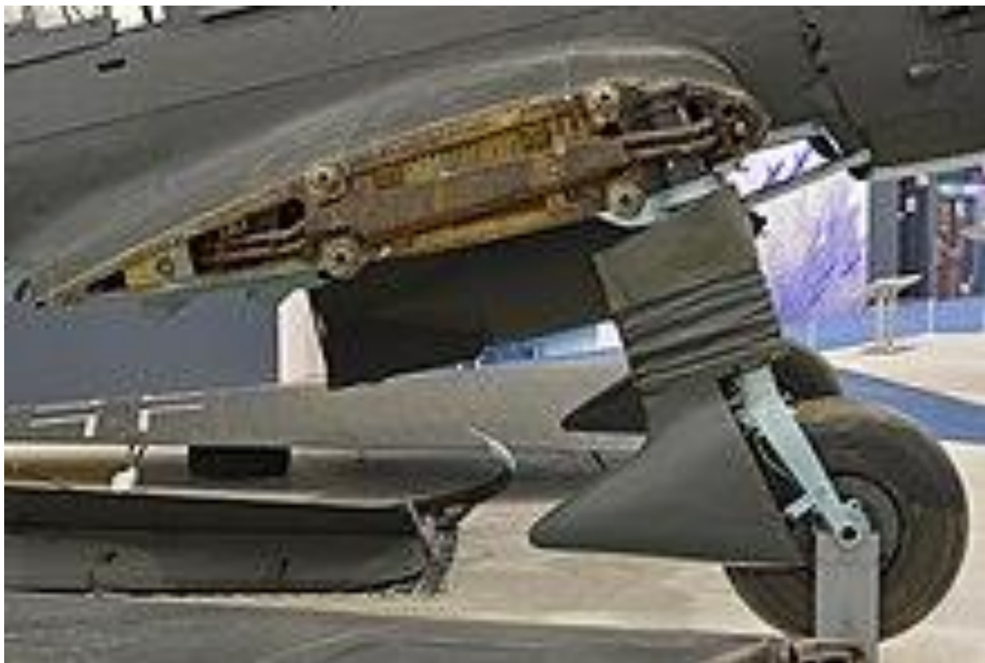
The RAF Museum's Ju 87, 2016, partially disassembled, showing the four attachment points for the outer wing section
