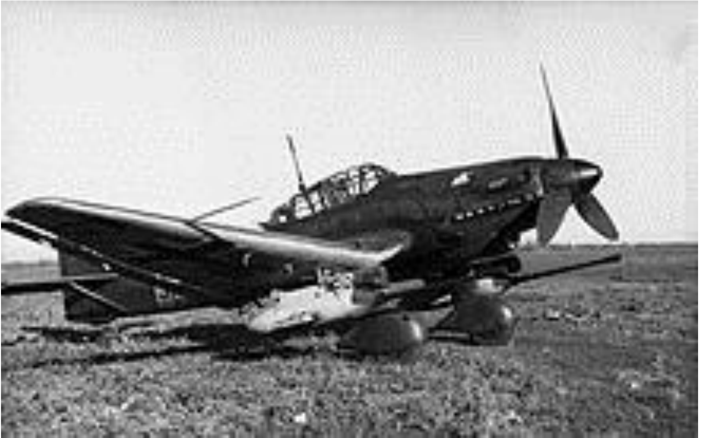
Ju 87 G-1 " Kanonenvogel " with its twin Bordkanone 3.7 cm (1.46 in) underwing gun pods
