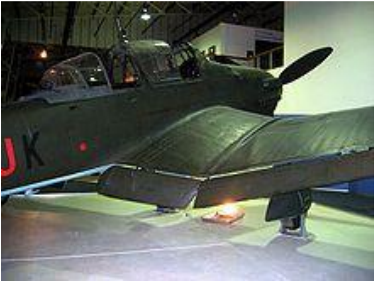
The Stuka had inverted gull wings, as shown in this photograph. Also visible are the two separate sliding "hoods" of the canopy.
