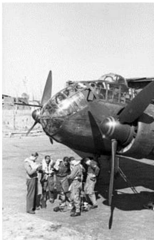
A view of the port side of the same machine, with Hohentwiel UHF radar aerials
