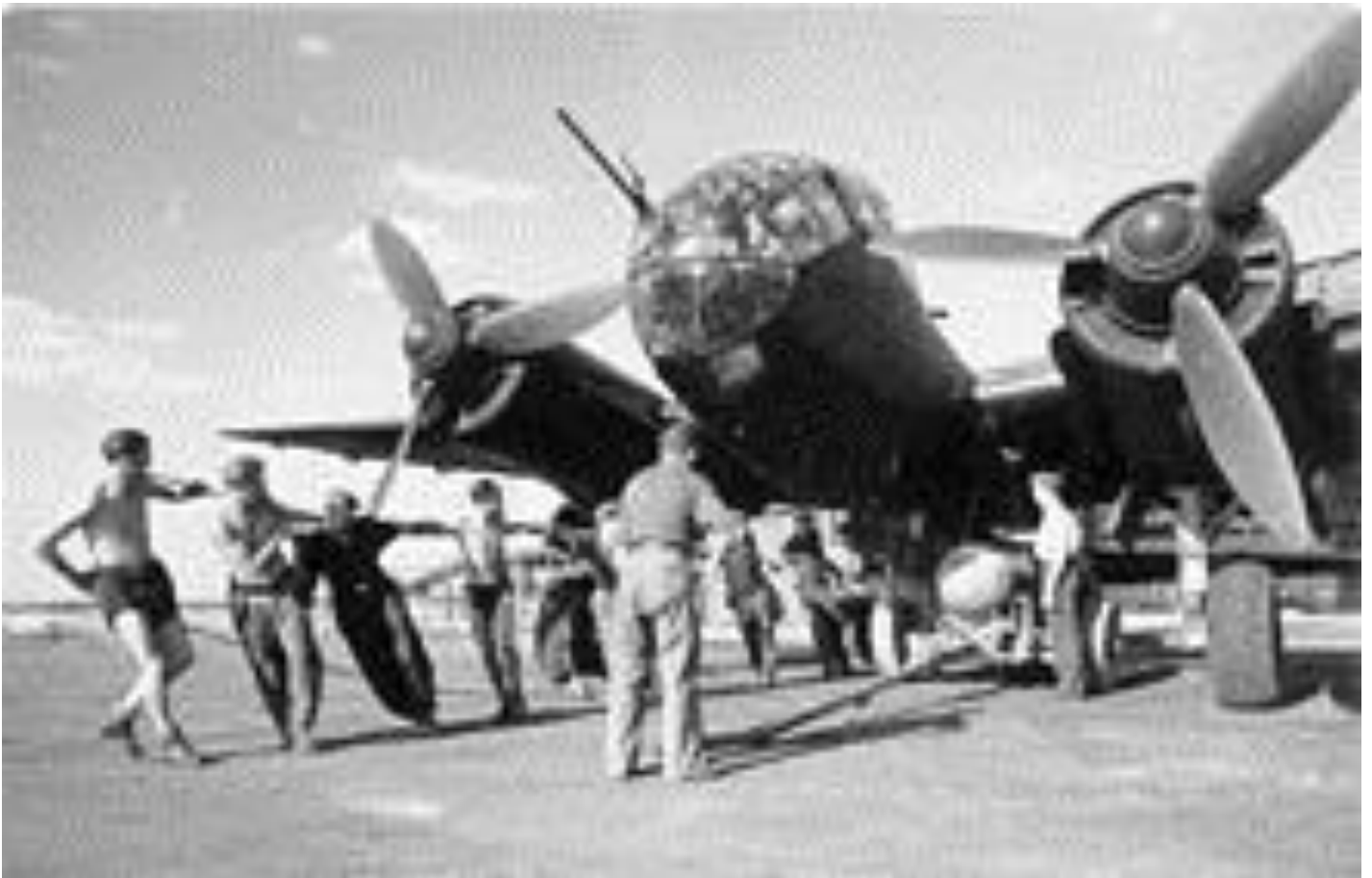
A Ju 188A-3 of Kampfgeschwader 6 being loaded with bombs. Western Europe, 1944 - note differing radiator core layout compared to that on the Ju 88A
