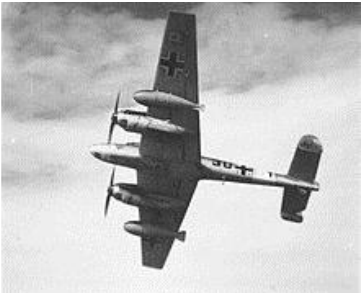
Bf 110 using standard 900-litre drop tanks, tested for the Do 217
