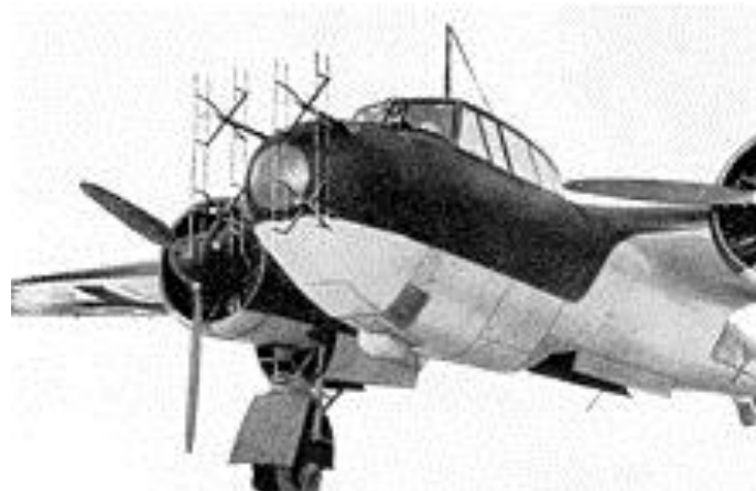
Nose of prototype Do 17 Z-10 Kauz II night fighter, similar to that of the Do 217 J, equipped with Matratze (mattress) 32-dipole radar antenna for its UHF-band early model Lichtenstein BC AI radar gear
