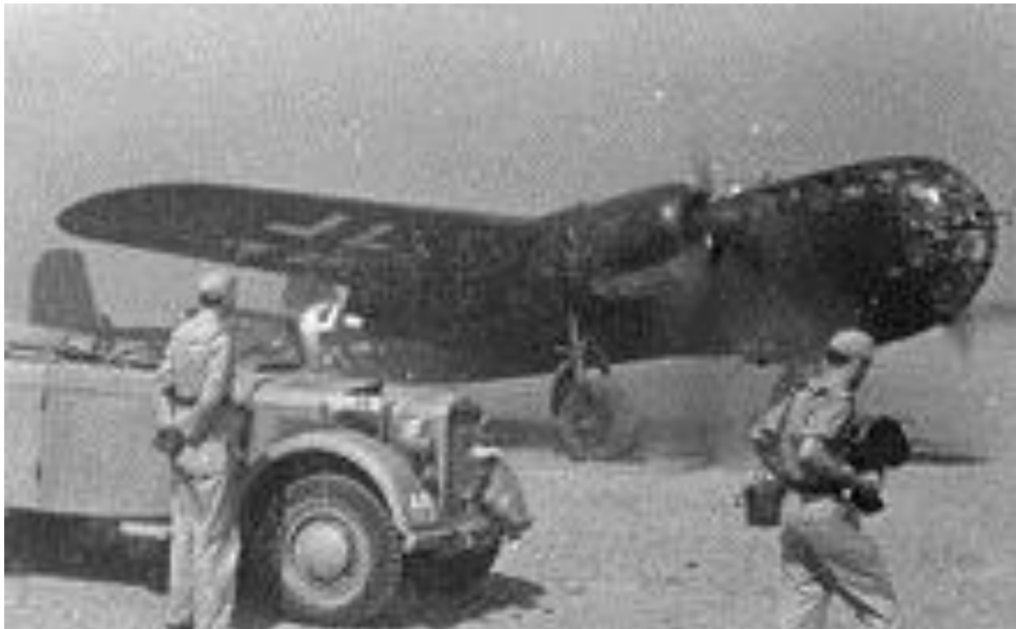
Do 217K-2, with the K-version's standard "stepless cockpit"
